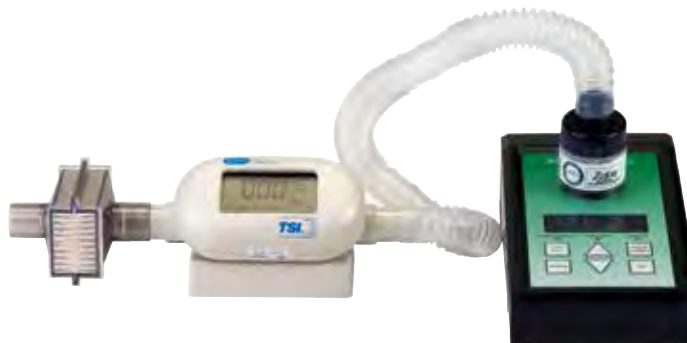
Bio-Pump® connected to a TSI Primary Flow Calibrator
